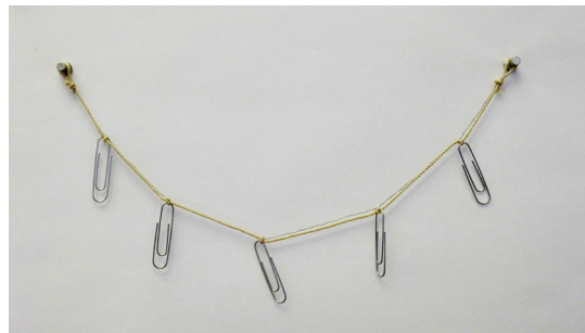
PHOTO 3: Testing how weight from paper clips changes the shape of a catenary curve
